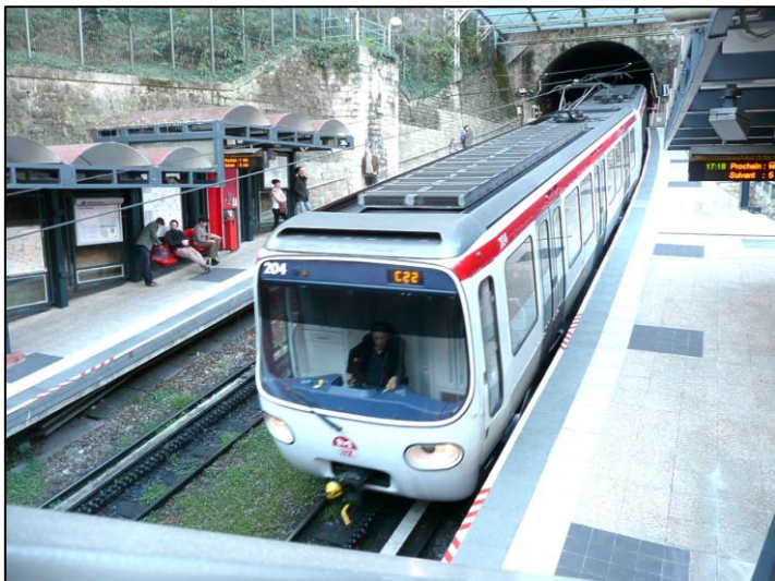
Ligne C train at the intermediate station (Croix-Paquet) on the rack section. Trains for Lignes A and B are similar but run on rubber tyres.
